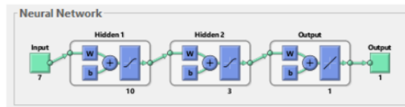
Figure 13 Structure of ANN developed using MATLAB
