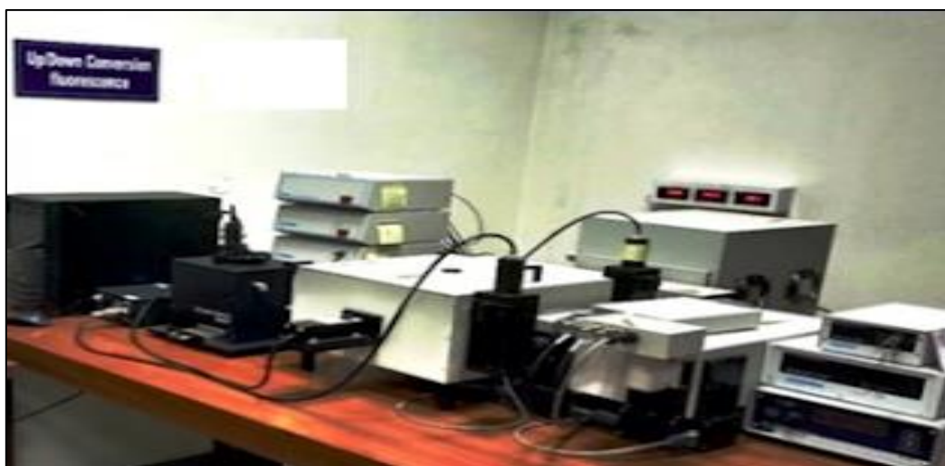
Figure 2.12: Upconversion luminescence spectroscopy Horiba PTI Quanta Master equipped using 980 nm laser
