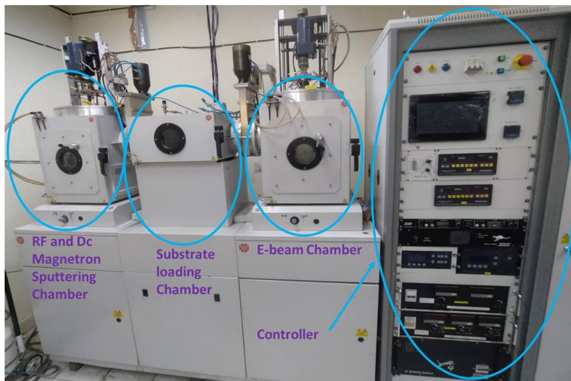
Fig.: 2.10 HHV-made Dual Beam (RF/DC magnetron sputtering) system
