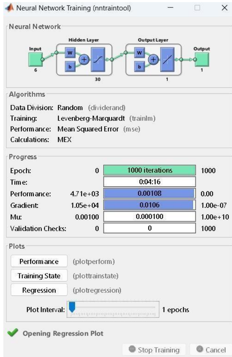
Fig. 4.3 showing training of AI for prediction of Base Shear
