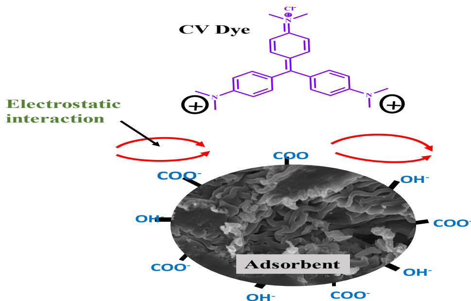
Figure 15. Mechanism of Adsorption on the adsorbent
