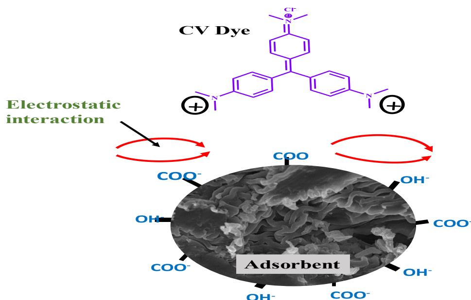
Figure 15. Mechanism of Adsorption on the adsorbent
