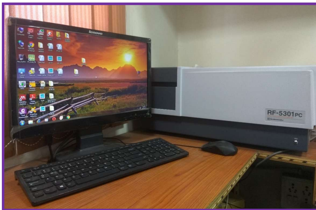
Fig. 2.17: Shimadzu, RF-5301PC spectrofluorophotometer connected with a computer.
