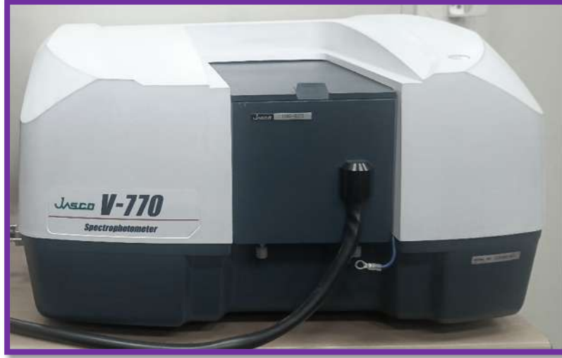
Fig. 2.11: UV-VIS spectrophotometer made by Jasco, model V770.
