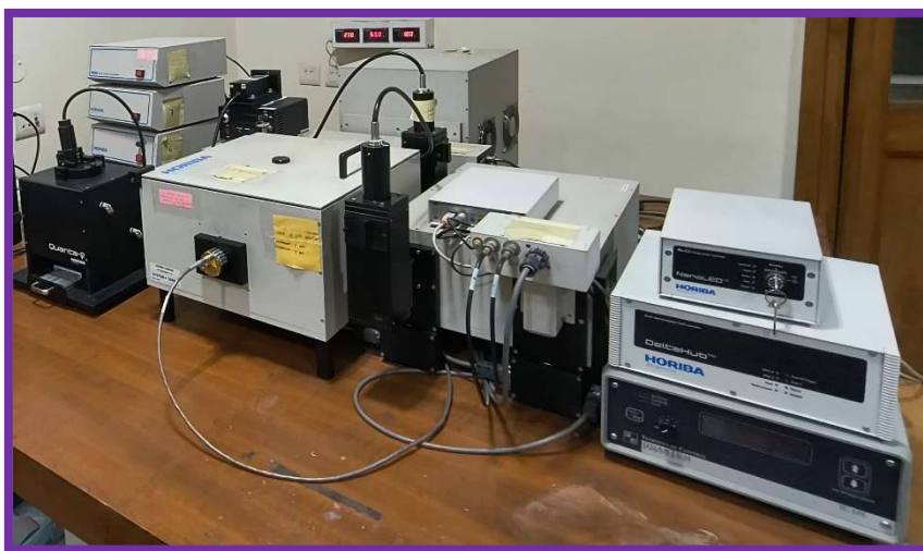
Fig. 2.18: Horiba PTI Quanta Master 8450-11 fluorometer .
