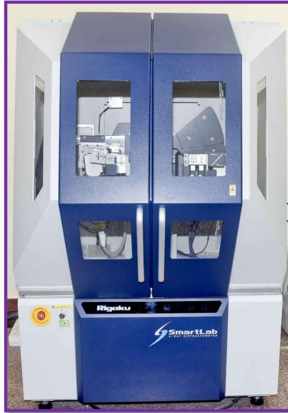
Fig. 2.09: Rigaku Smart lab advance X-ray diffraction machine.
