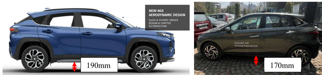
Figure 61: Ground Clearance for Fronx and I20 (Source: NexaExperience, n.d.)
