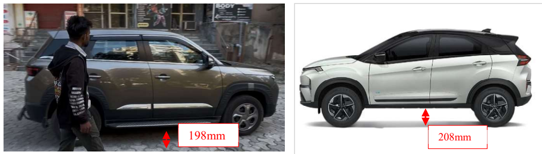
Figure 34: Ground Clearance (Source: Tatamotors, n.d)
