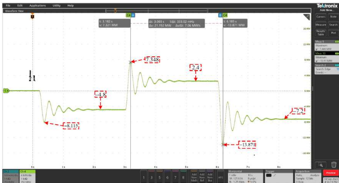
FIGURE 3.21: Frequency deviation (a) 5MW, (c) 7.5MW, (e) 10MW. Power change (b) 5MW, (d) 7.5MW, (f) 10 MW
