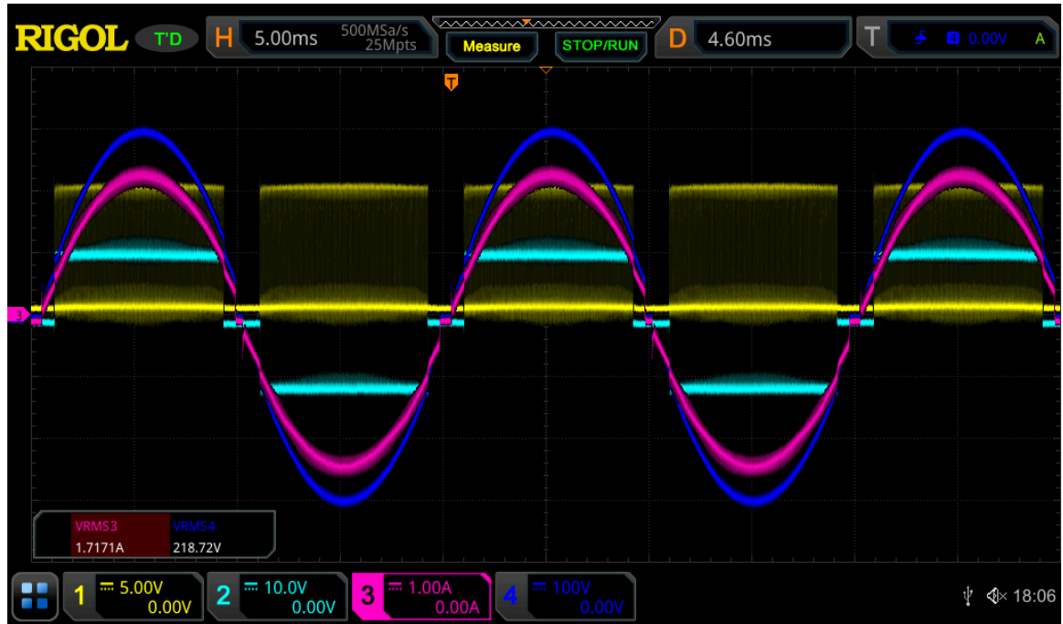
Fig. 7.5 Sinusoidal Pulse Width Modulation of Voltage Source Inverter
