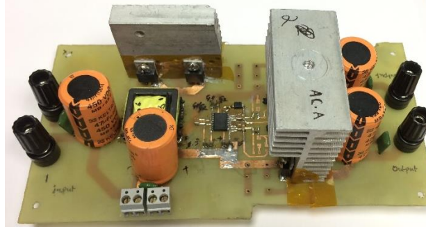
Fig 3.10 Hardware Prototype of Proposed Impedance Converter
