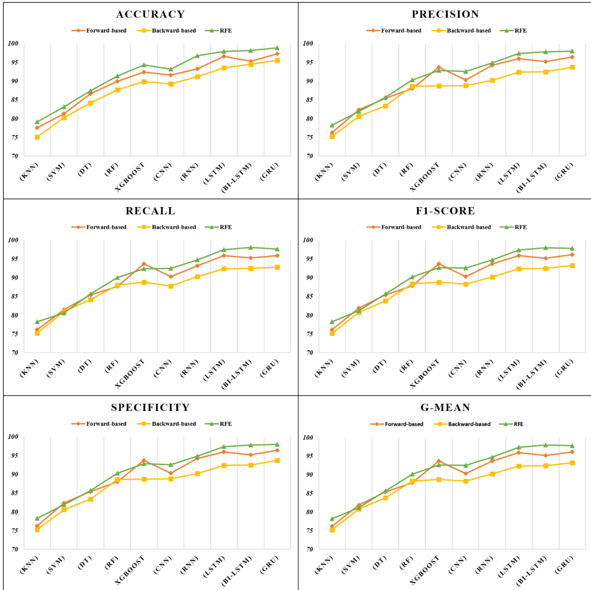
Figure 7.20: Comparison of AI-based IDS models on different Wrapper-based Feature selection methods using the N_BaIoT dataset.
