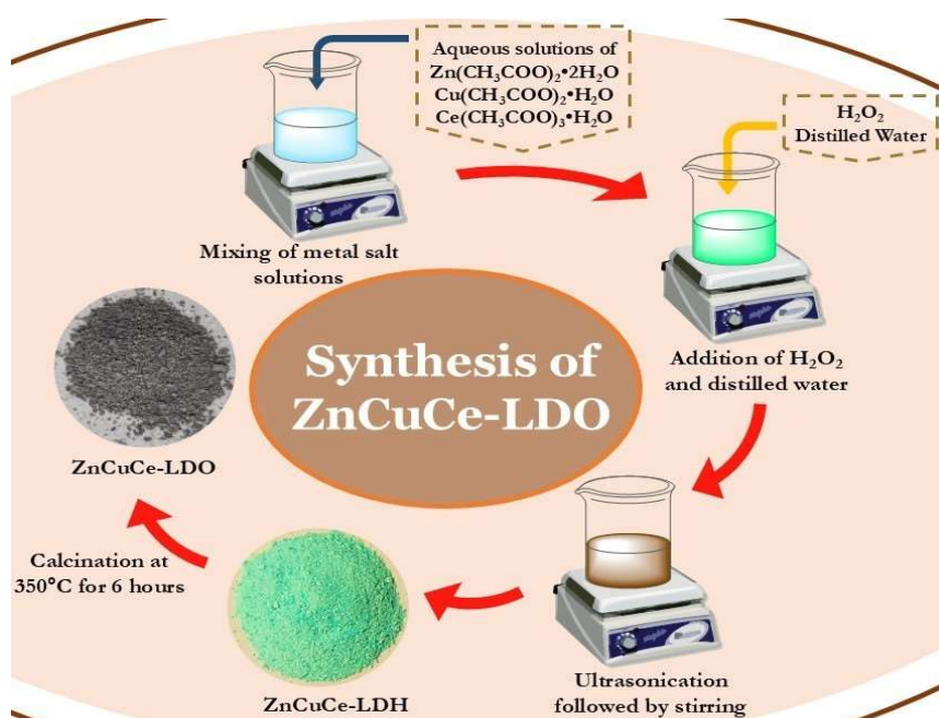
Figure 4.1 Synthesis of ternary ZnCuCe-LDH and ZnCuCe-LDO.
