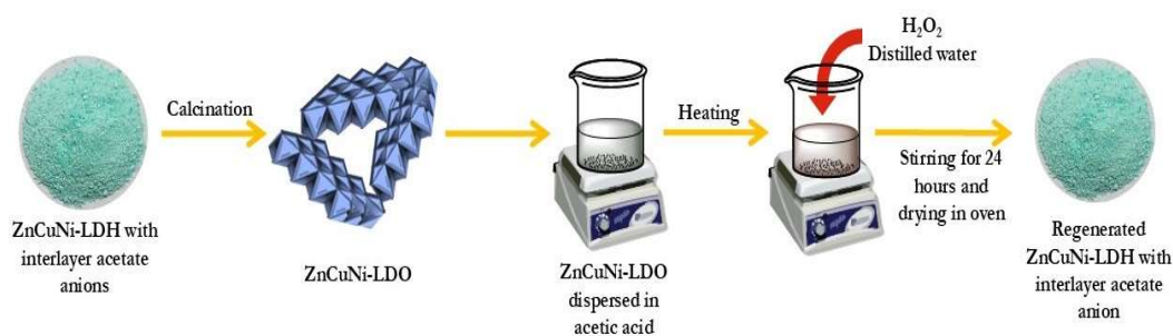
Figure 5.2 Schematic representation of the calcination-regeneration process for demonstrating memory effect property of LDHs.
