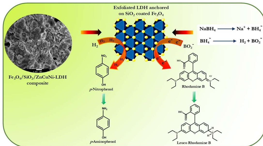
Figure 7.11 Postulated mechanism for the \text{NaBH}_4 -assisted catalytic degradation of p -NP and RhB using \text{Fe}_3\text{O}_4/\text{SiO}_2/\text{ZnCuNi-LDH} composite.
