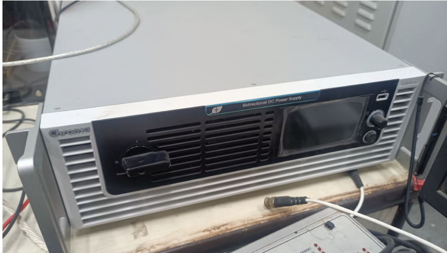
FIGURE 3.14: Bi-Directional DC power supply
