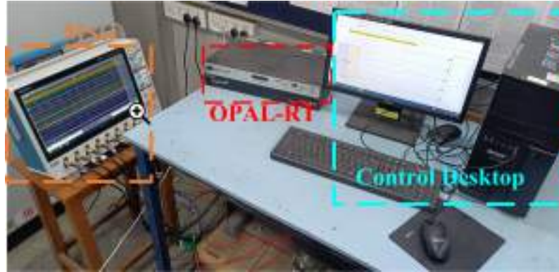
FIGURE 3.21: Real-time simulation setup
