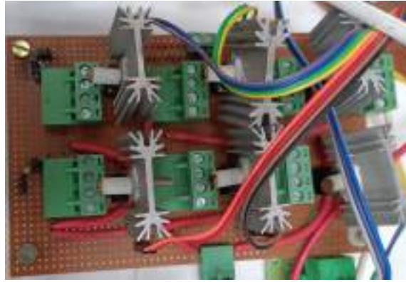
FIGURE 3.16: Hardware setup for AC/DC converter
