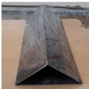
Figure 3.2 (a) Definition sketch of experimental setup; (b) Definition sketch of strip macroroughness; (c) Physical strip macroroughness elements
