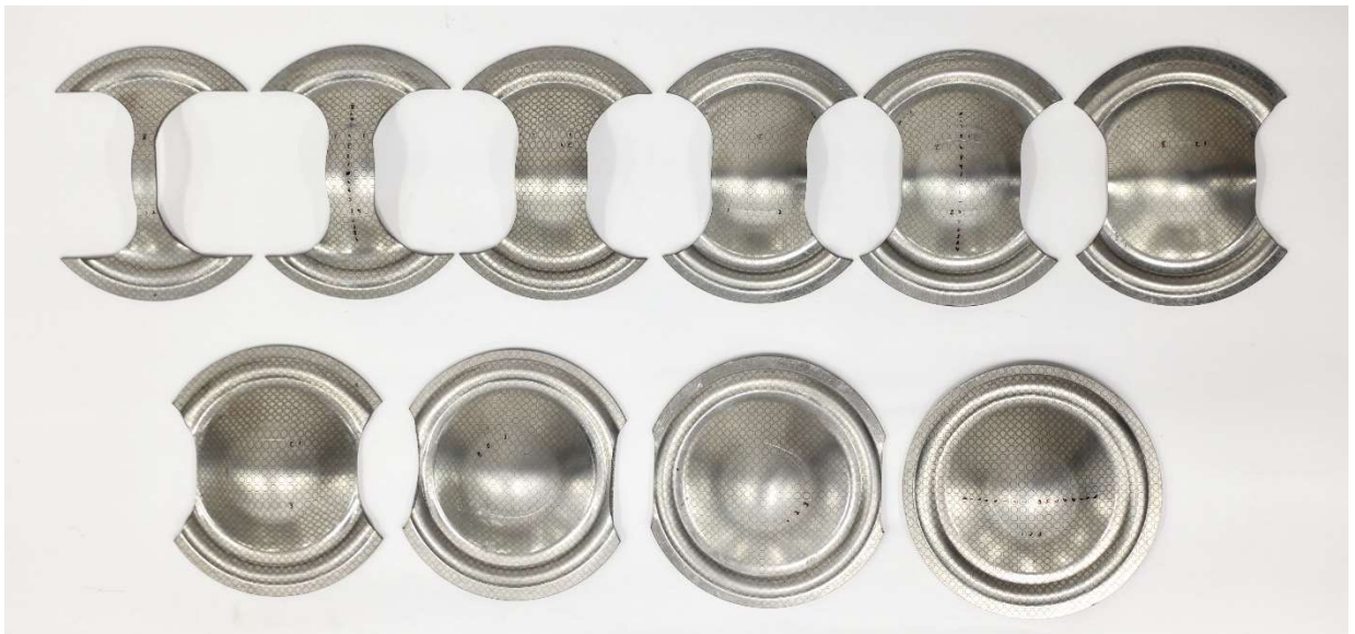
Fig. 6.18. Test FLD specimens of 2-ply clad sheet with steel as outer layer of dome
