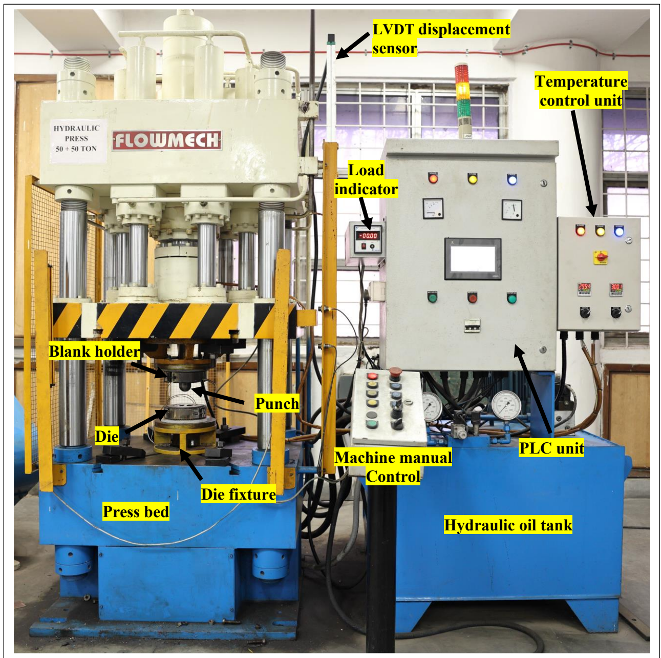
Fig. 5.16 Experimental setup showing assembly of fabricated tools integrated with 100 tonne capacity hydraulic press
