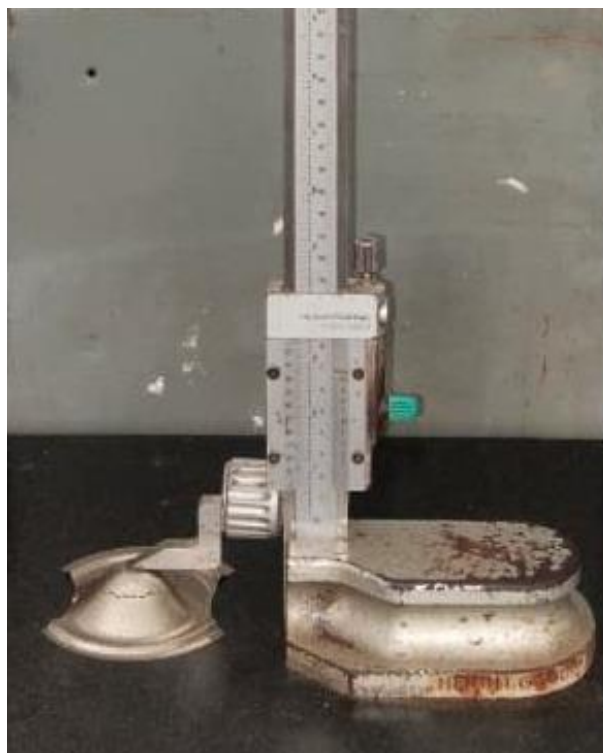
Fig. 5.22 Dome height measurement of FLD specimen using vernier height gauge
