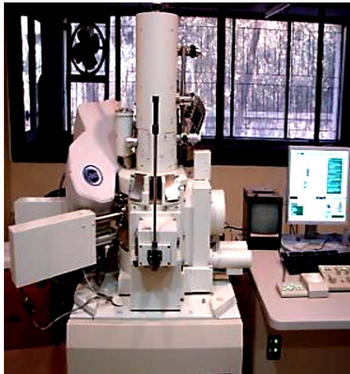
Fig. 5.24 Field emission gun (FEG) scanning electron microscope (SEM) for electron backscattered diffraction (EBSD) analysis
