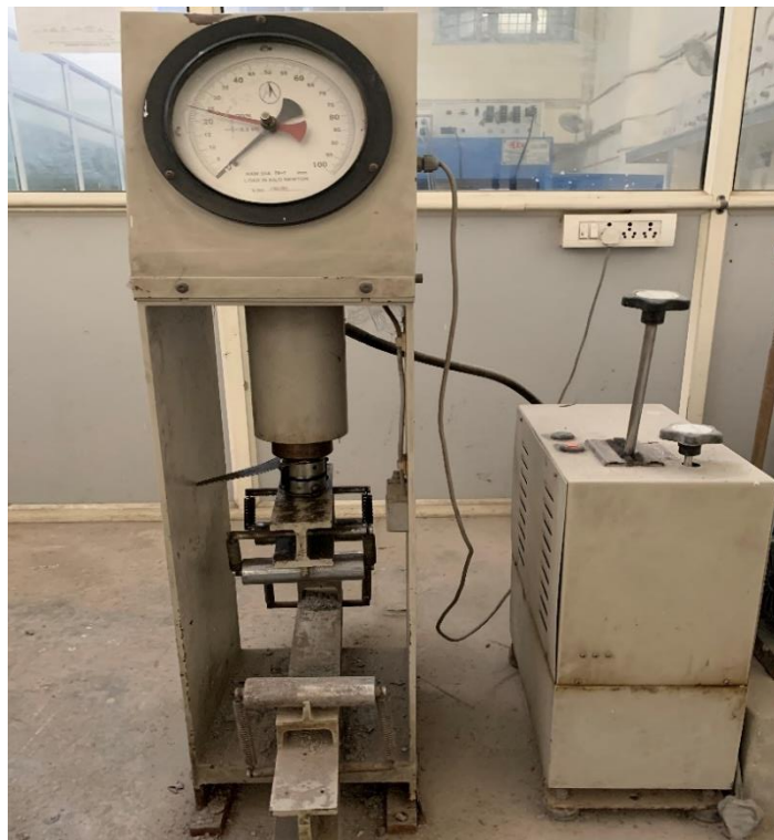
Fig. 3.13: The flexural strength test setup
