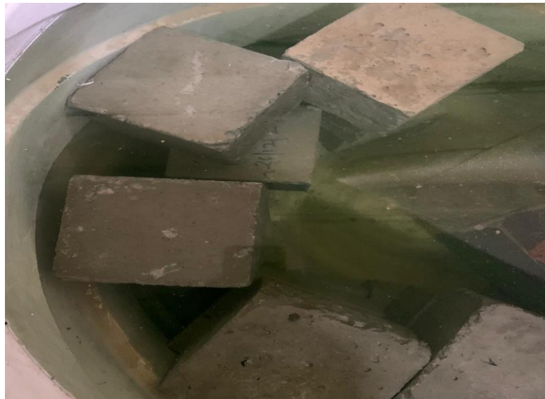
Fig. 3.15: Picture of seawater solution with the cube specimens
