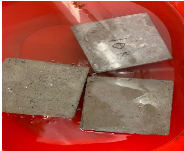
Fig. 3.16: Picture of sulphate solutions with the cube specimens
