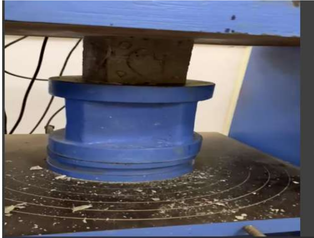
Fig. 3.12: Compressive Strength Test of GPC Cube in the CTM
