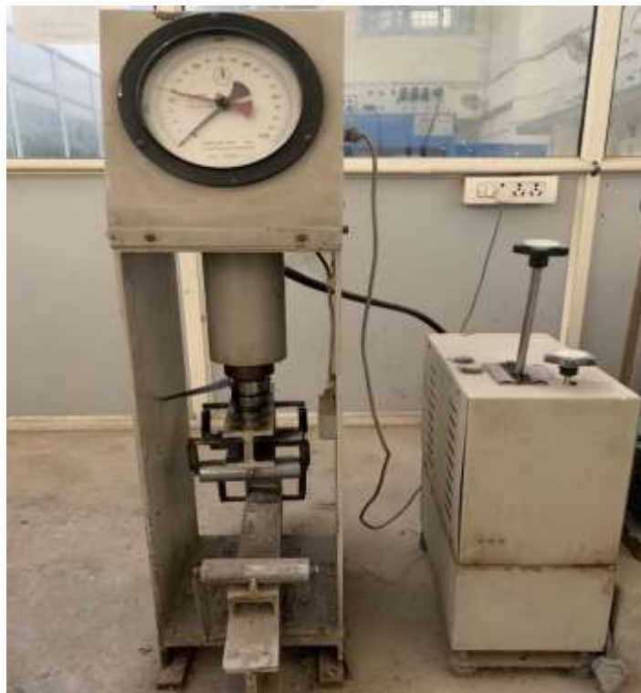
Fig. 3.13: The Flexural Strength Test Setup
