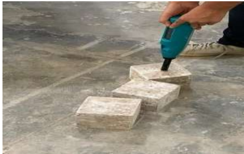
Fig. 3.14: Picture During Rebound Hammer Strength Test
