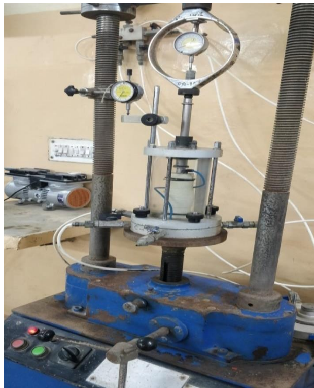
Fig 3.13 Triaxial shear test apparatus
