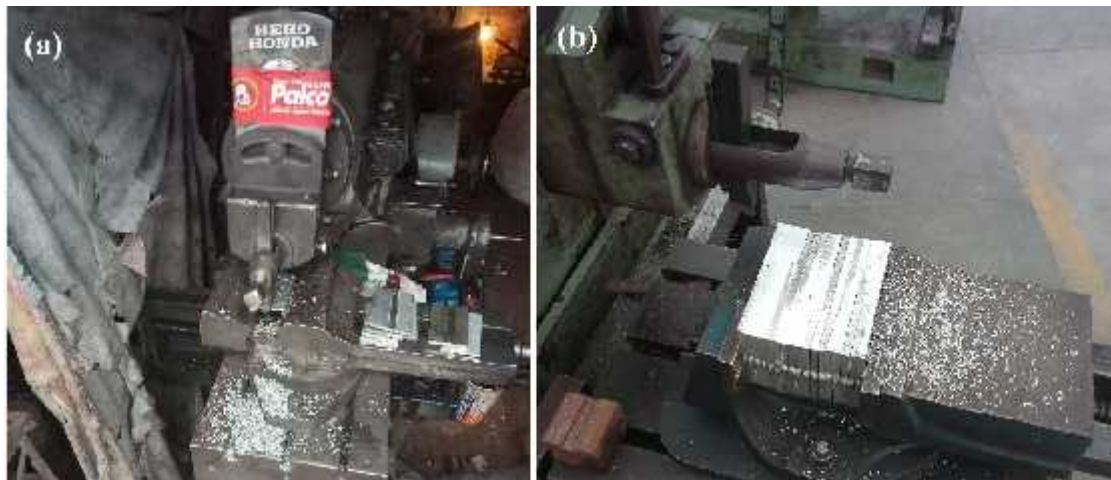
Figure 39: (a) Removal of weld bead by shaper machine, (b) finishing of the welded plate
