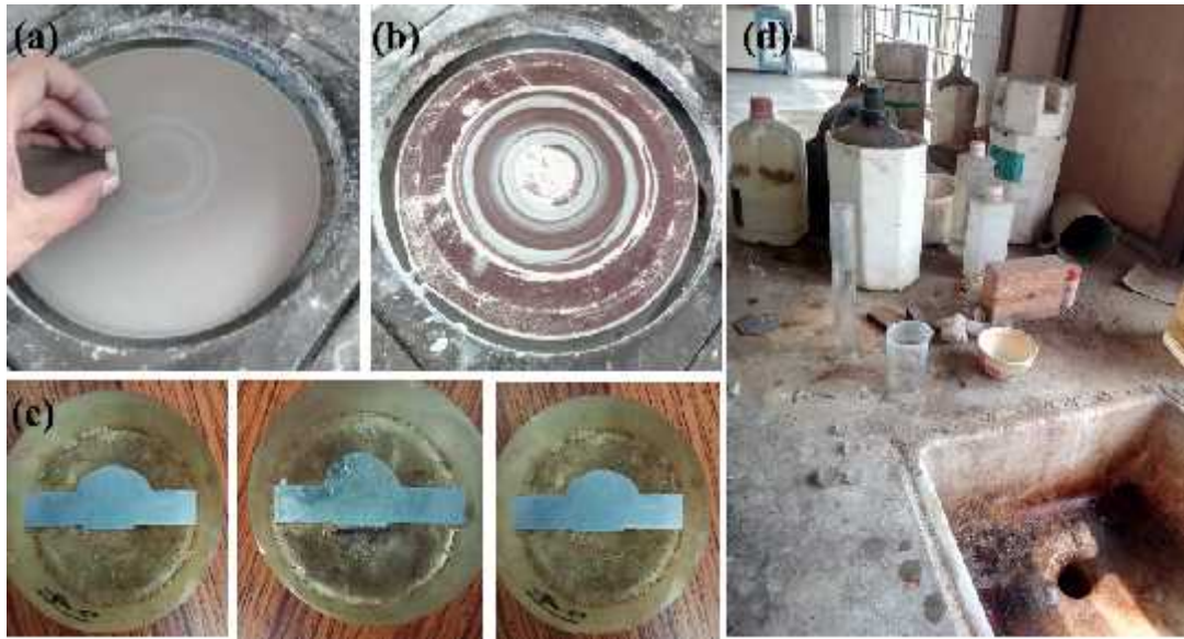
Figure 44: (a) polishing with emery paper, (b) polishing with emery cloth with \text{Al}_2\text{O}_3 powder, (c) specimen after polishing, (d) making etching solution
