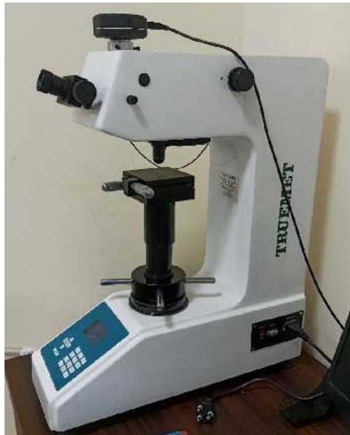
Figure 42: Vickers micro hardness testing process
