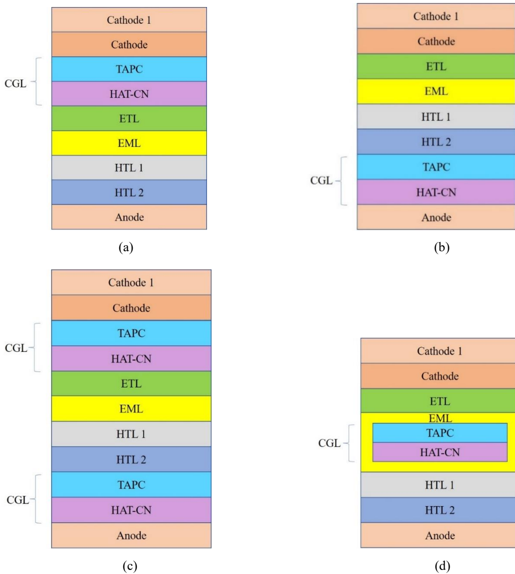
Fig. 4.4 Different OLED structures based on positional variation of CGL (a) Below cathode (L 2 ), (b) Above anode (L 3 ), (c) Both sides of device (below cathode and above anode) (L 4 ), and (d) Inside emissive layer (L 5 )
