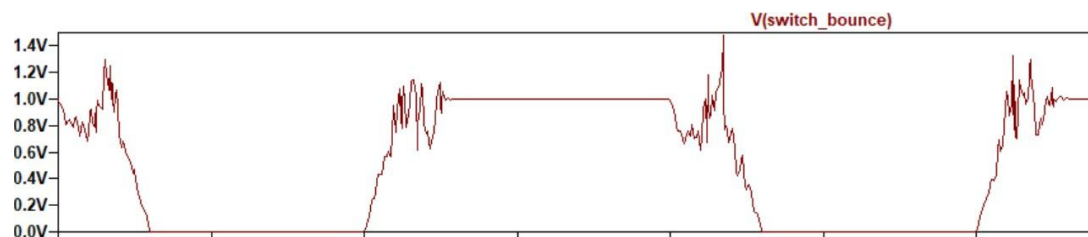
Fig. 3.2:- Input switch bounced signal
