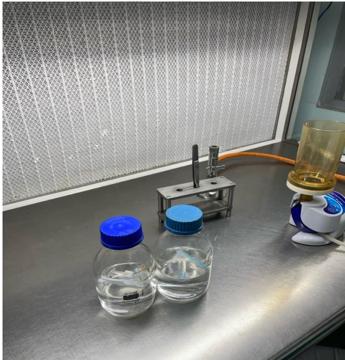
Figure 4.4. Sonication of a medical device in neutralizing buffer for microbial extraction.
