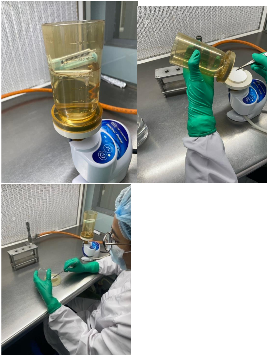
Figure 4.6. Filtration of extracted sample and placement of membrane on TSA plate.
