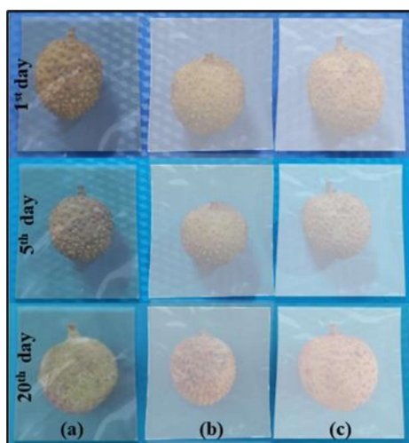
Fig. 5.10 Litchi Preservation performance of (a) Polyethylene film, (b) PLA/PEG film and (c) PLA/PEG/PBAT film
