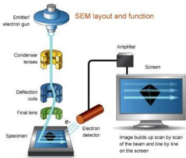
Fig. 3.4 Schematic diagram of SEM
