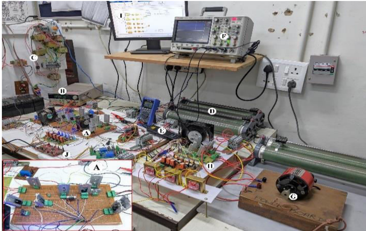
Figure 5.14. Laboratory setup for converter's prototype: (A) Proposed MIMO converter, (B) Input power supply for sources and ESE, (C) Controller and sensor power circuit, (D) DC Resistive Load, (E) Probes for measurements, (F) Digital Storage Oscilloscope and (G) Motor Setup (H) Inverter Configuration (I) Computer setup (J) TMS320F28379D DSP.
