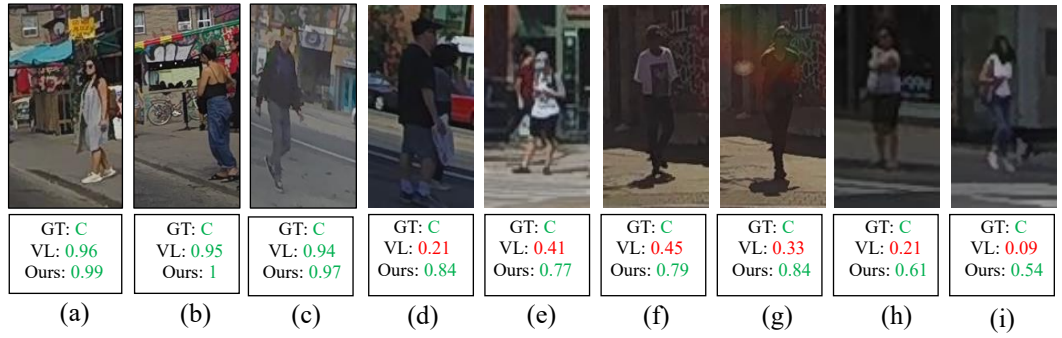
Fig. 3.22: Qualitative predictions on PIE/JAAD where IntentFormer correctly classifies intent, unlike the vanilla transformer. Red: non-crossing, Green: crossing.
