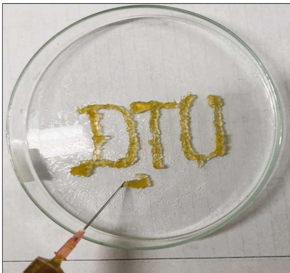
Fig. 6. 3 Injectability evaluation of synthesized injectable hydrogel
