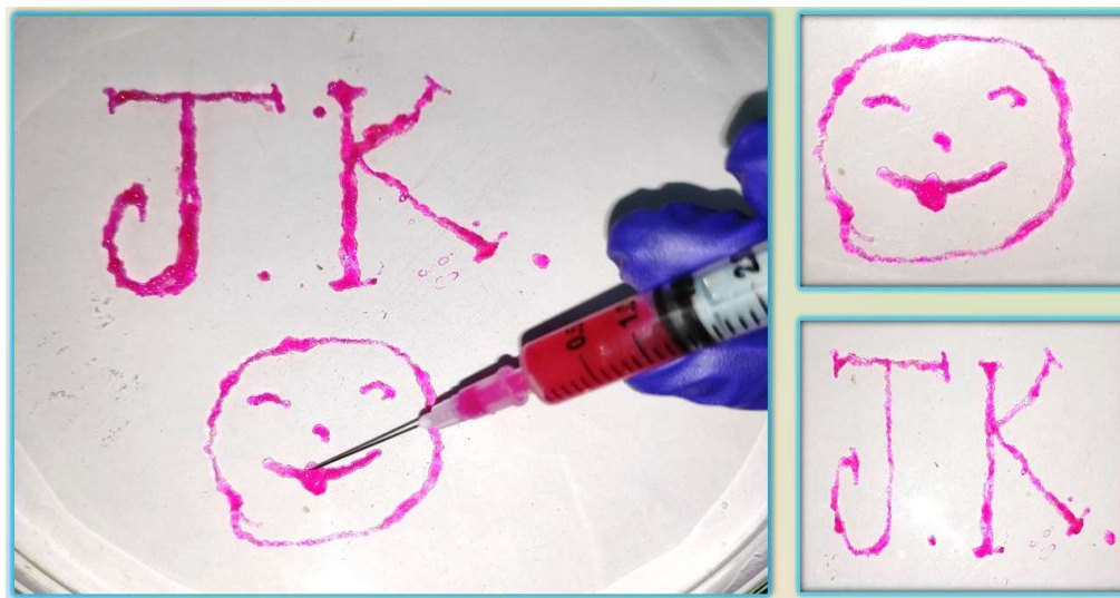
Fig. 7. 2 Injectability evaluation of OG2C1 using 26 G needle.
