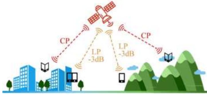
Fig .2.8 A Polarization Reconfigurable Antenna for Satellite application [28]
