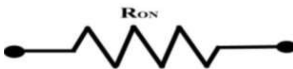
(a) ON state equivalent lumped element
