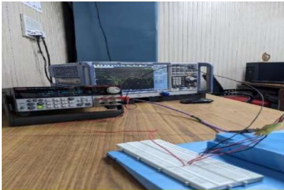
(a) S-parameter measurement
