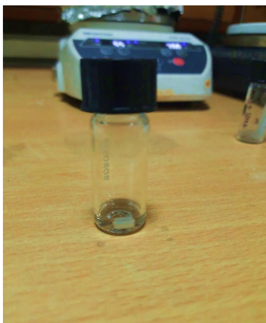
Figure 9: Tartaric acid–imidazole DES prepared via heating and mixing
