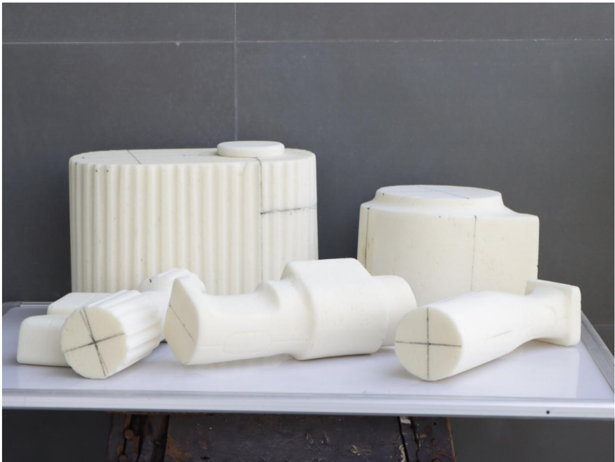
Figure 4.14. Collection of PU foam models used to test and visualize finalized concepts
