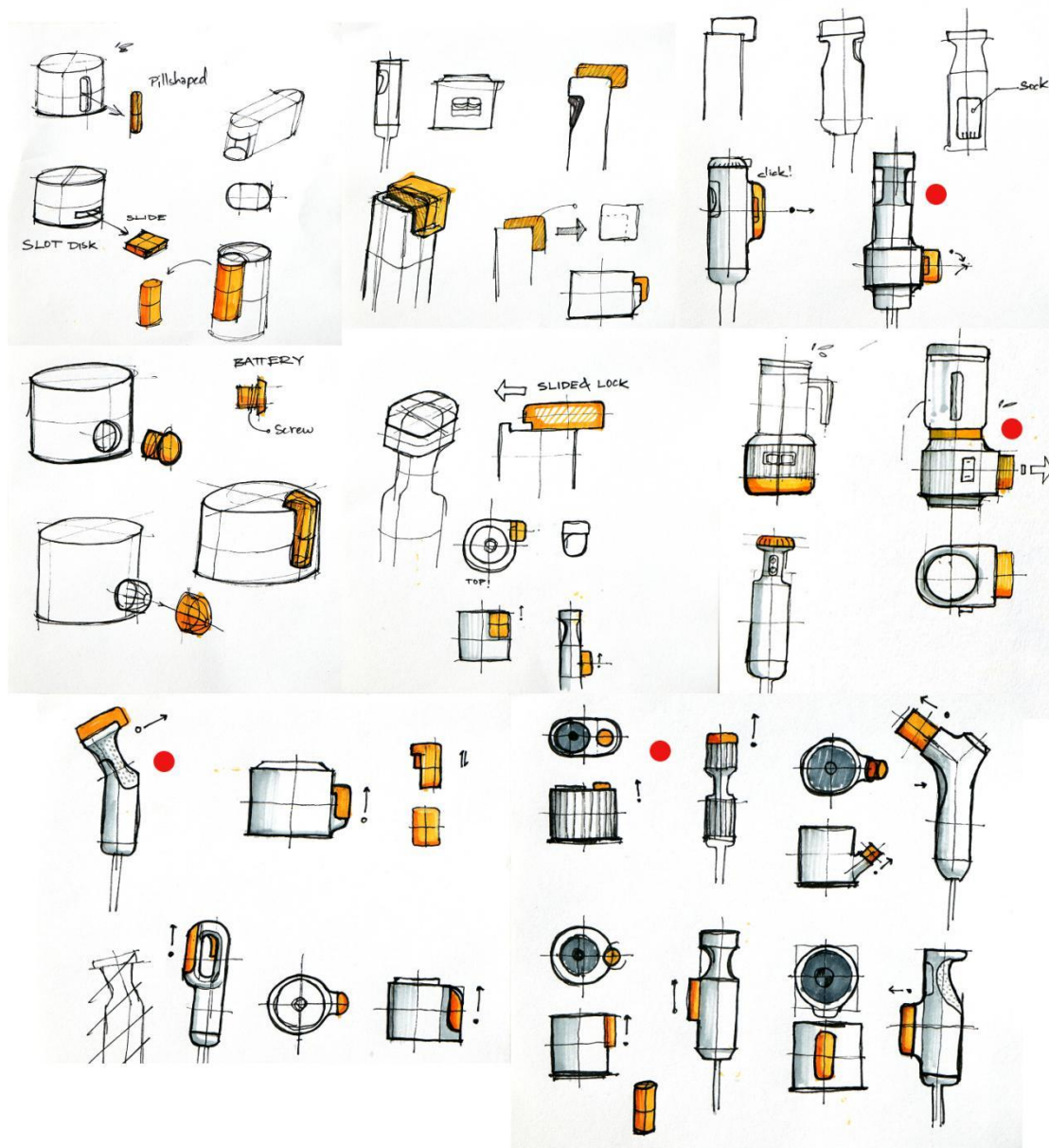
Figure 4.8. Form ideation sketches: showcasing different options for battery attachment and form of the appliances
