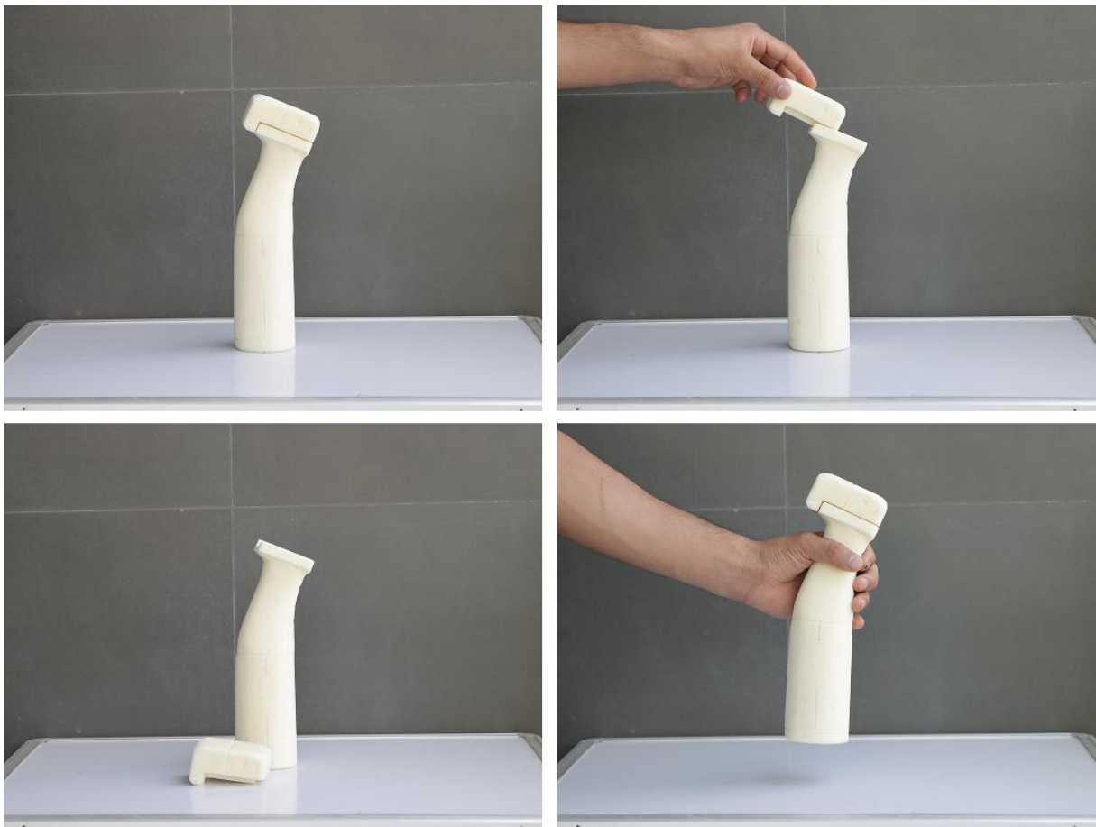
Figure 4.16. Series of images of PU foam model of Concept 2 - Ergonomic grip curve
