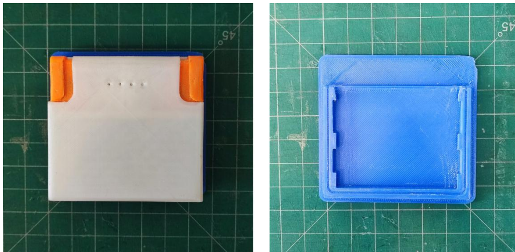
Figure 5.7. 3D printed models of battery and slot with working attachment mechanism
