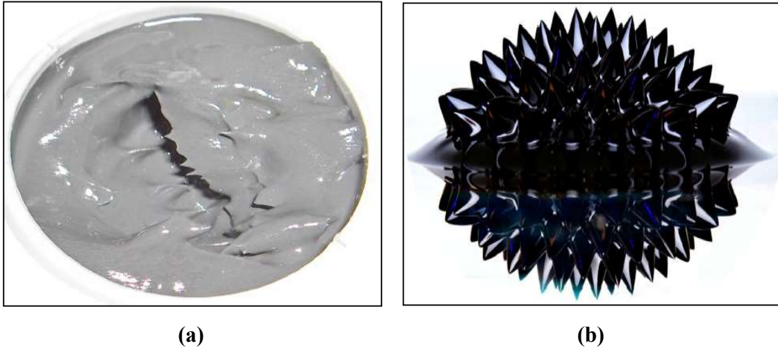
Fig. 8: (a) Magnetorheological fluid with no magnetic field (b) Ferro fluid in presence of magnetic field [15]
