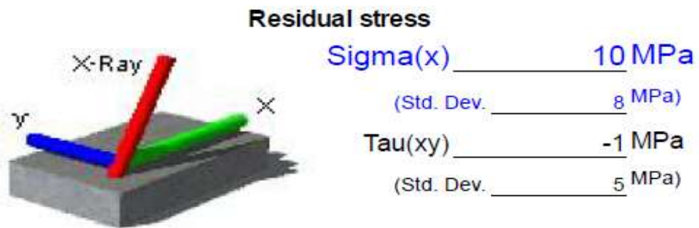
Fig. 42: Residual stress on Al7075 workpiece surface after BEMRF process
