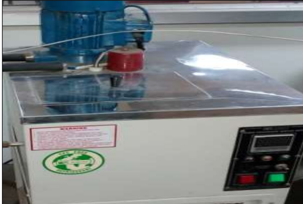
Fig. 25: Chiller for cooling the electromagnetic coil
