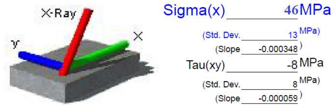
Fig. 41: Residual stress on Al7075 workpiece surface after grinding process
