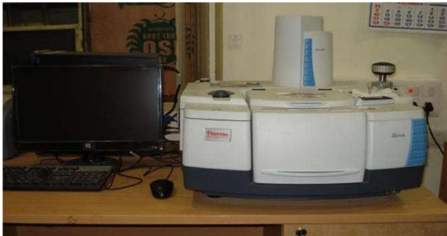
Figure 19: Setup of Nicolet iS50 FTIR Tri-Detector.
