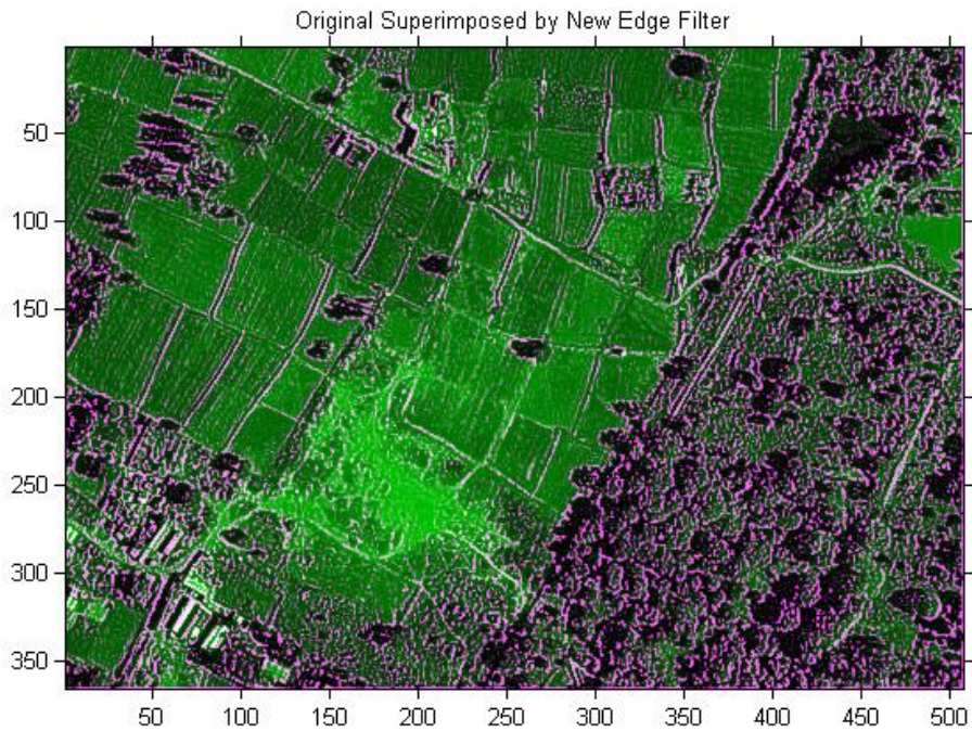
Fig. 5.8 Original image superimposed by proposed edge filter
