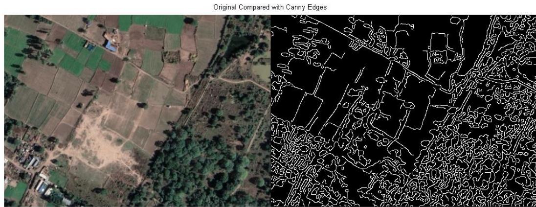
Fig. 5.9 Original image compared with Canny Edges
