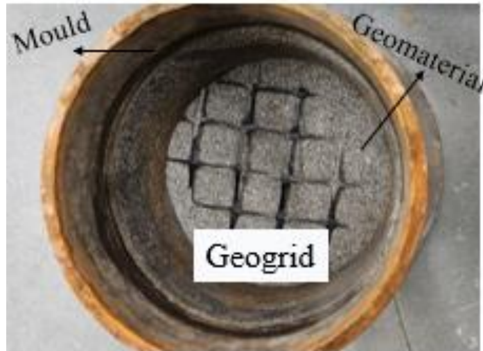
Figure 13: Pictorial representation of the geomaterial reinforced with geogrid placed inside CBR mould before soaking for 96 hours
