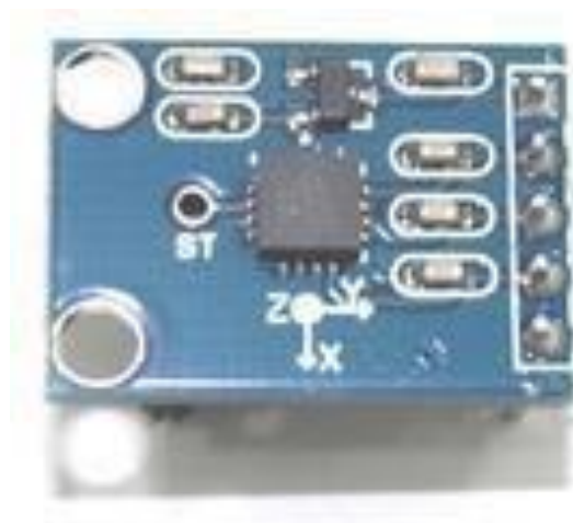
Fig.3: Accelerometer GY-61 ADXL335 3-Axis Accelerometer Module
