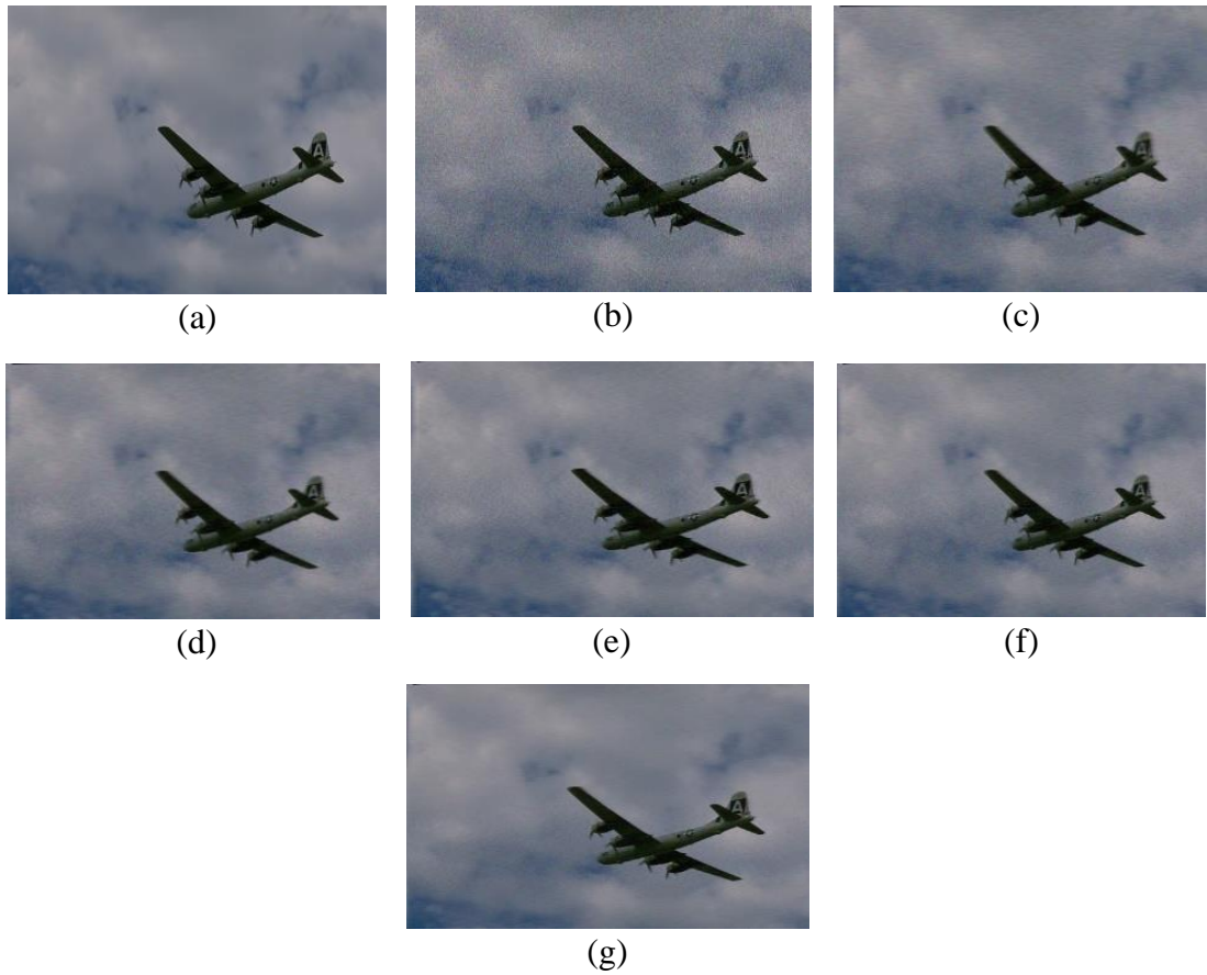
Fig. 5.3 Visual Comparison of Denoising Performance. (a) Clean Ground Truth. (b) Noisy input ( \sigma = 15 ). (c) LMS output. (d) Lncosh output. (e) VSLMS Ang's output. (f) Fusion-Based Filter output. (g) Bilateral + Fusion Filter output.
