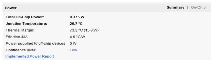
Figure 4.6 Power Utilization report after synthesis for DHT
