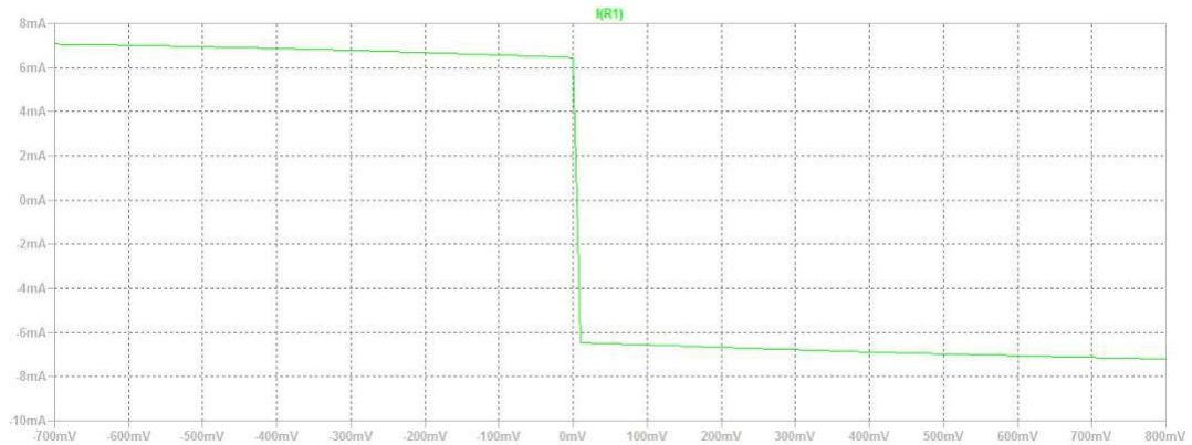
Fig. 2.3: I-V characteristics of AD712 Opamp
