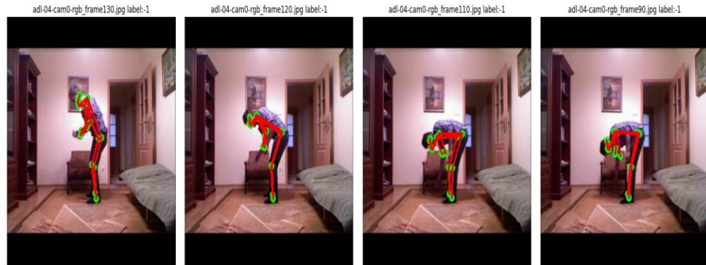
Fig.6.3 Extracted Skeletal Keypoints of frames in ADL sequence along with their Label.
