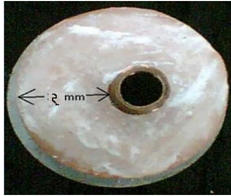
Figure 4.1: Copper vortex tube with wax casting and covered by wooden material
