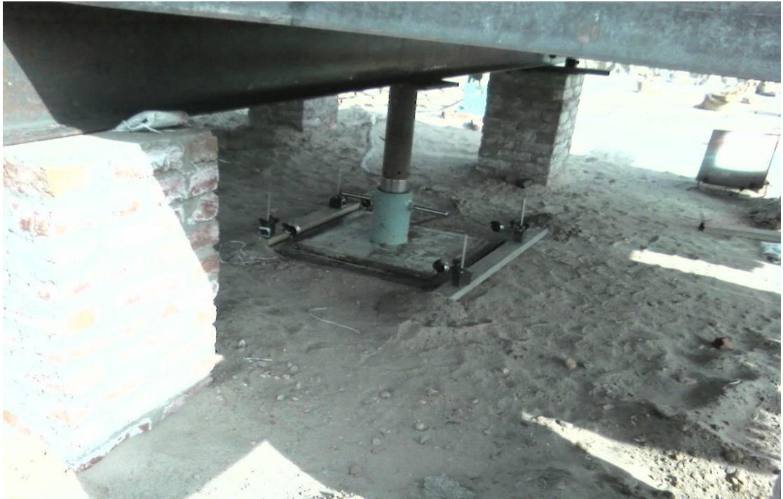
Photo 5.1 Plate load test setup at site
