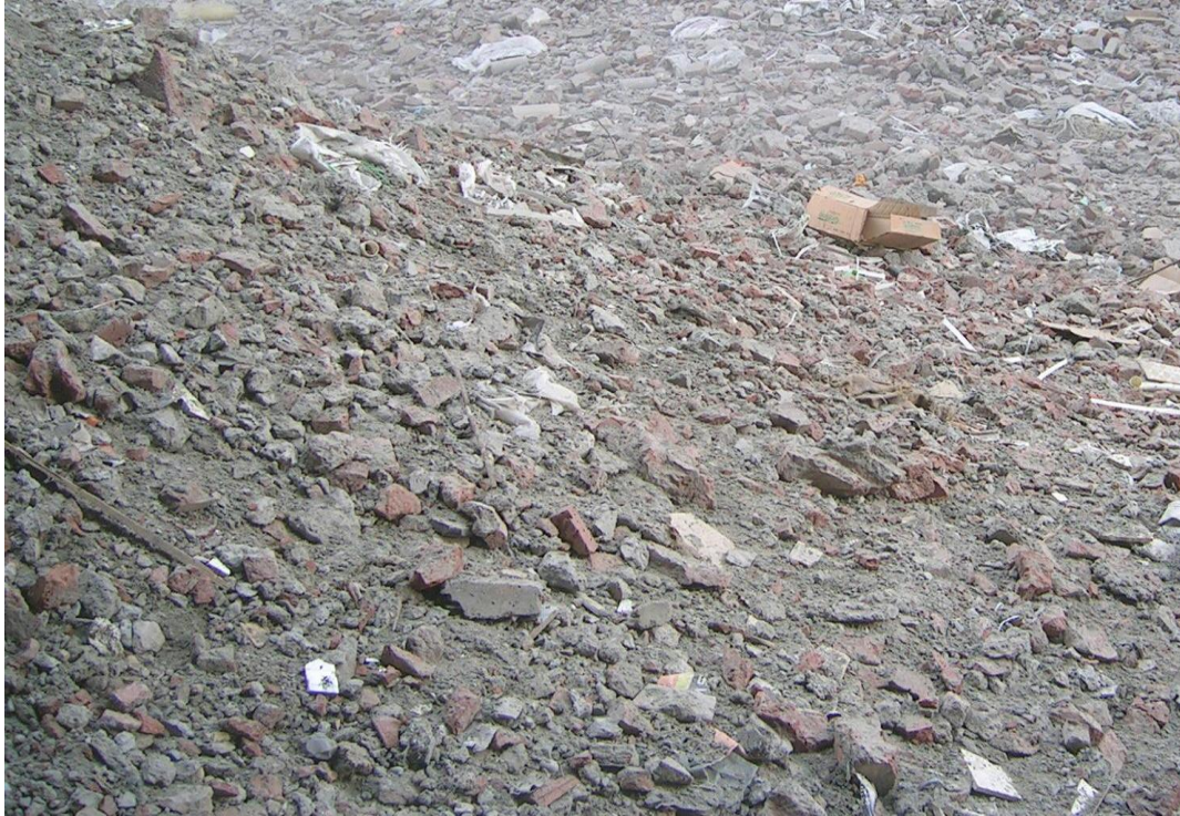
Photo-1.2 Construction waste consists of dry mortar and brick bats
