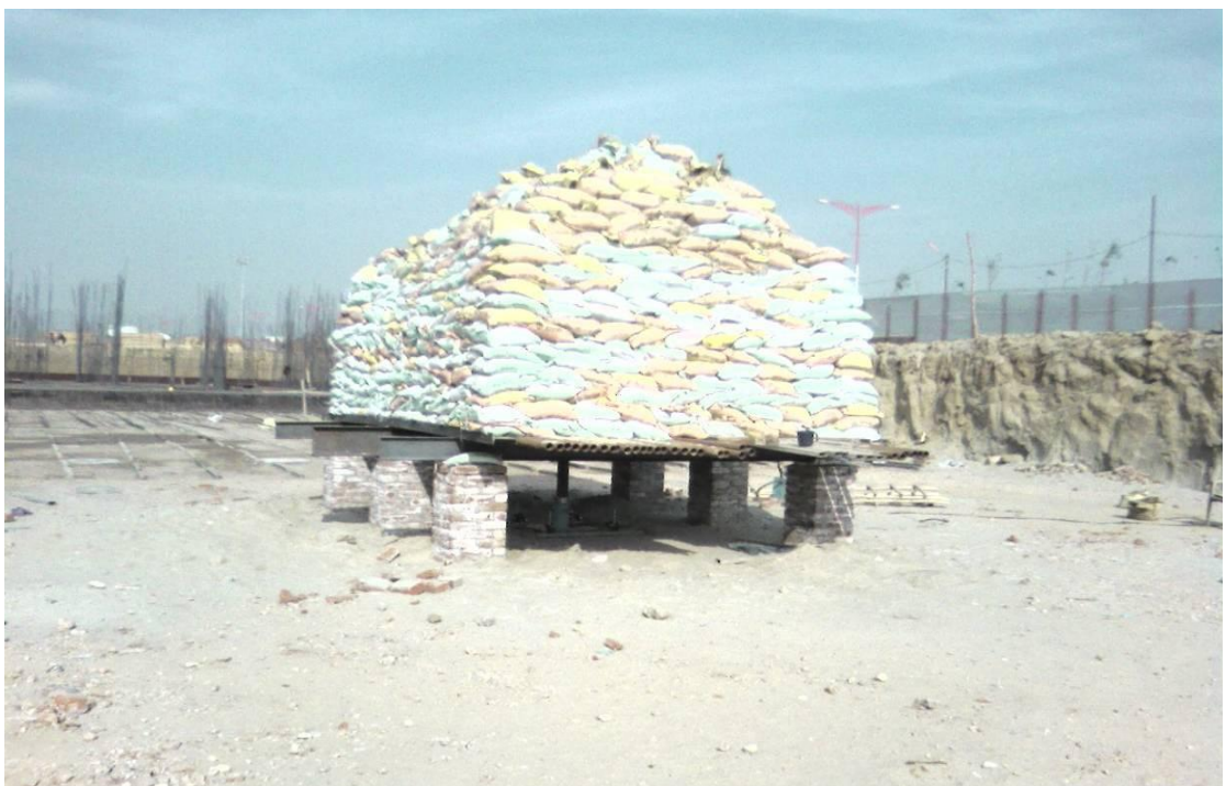
Photo 5.2 Plate load test setup at site
