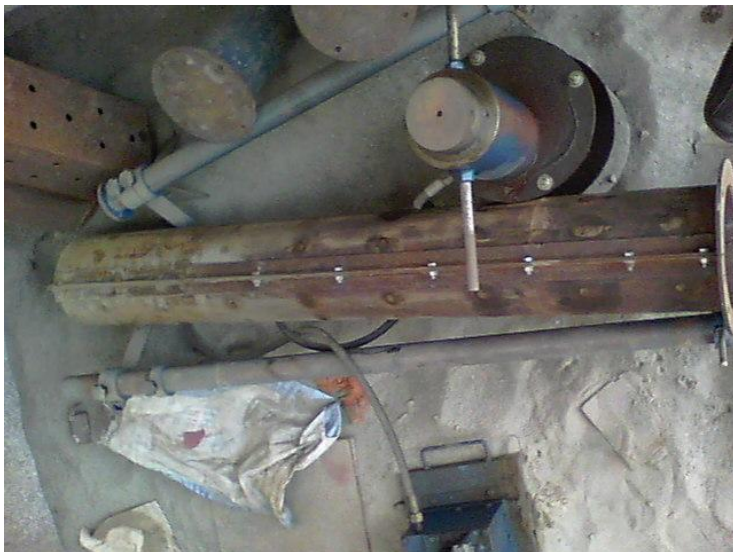
Photograph 25: Two halves were being nut-bolted through Welded angled-iron.
