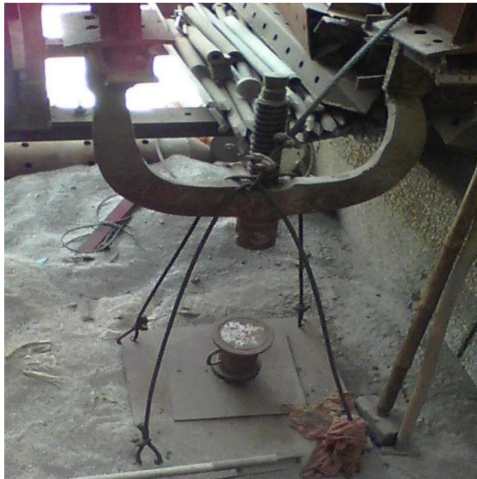
Photograph12: Lifting support mechanism, top tightening through vertical rotating assembly
