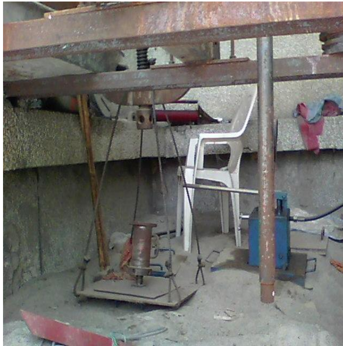
Photograph 13: Pull-out load arrangement through hydraulic jack, pump, lifting support mechanism
