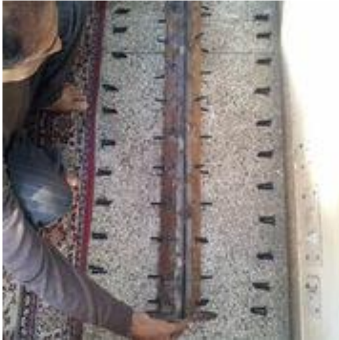
Photograph 15: Spikes arrangement for a model steel pile on a medium scale (not a part of this thesis) (View 1).
