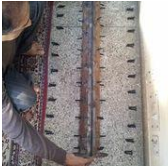
Photograph 16: Zig - zag spikes arrangement (Horizontal) for a model steel pile on a medium scale (not a part of this thesis). (View 2)
