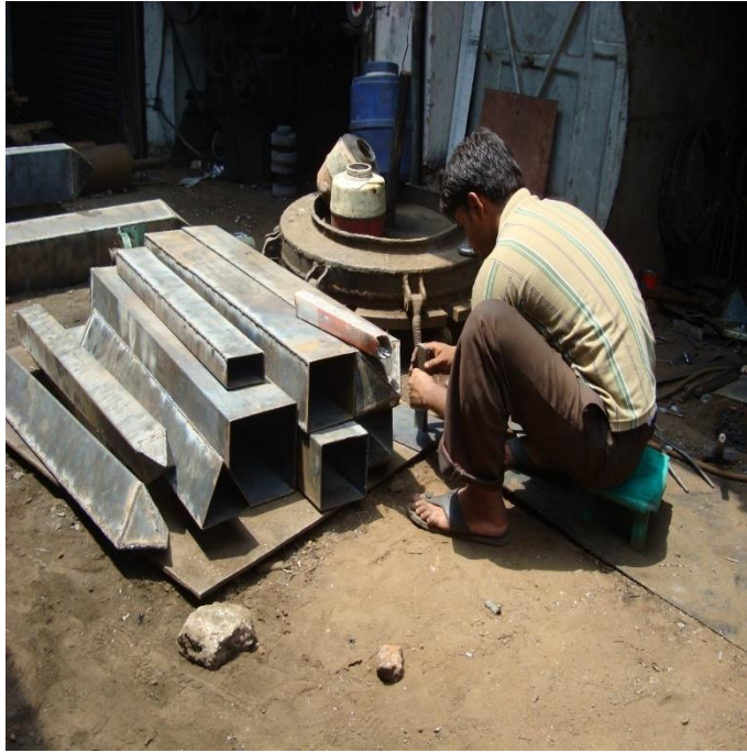
Photograph 7: Steel piles being fabricated at the machine lathe shop.
