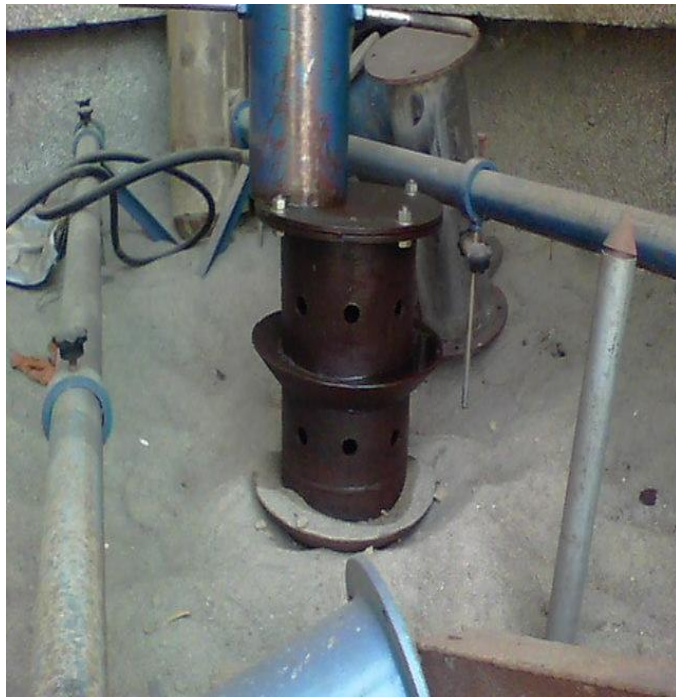
Photograph 20: Doubly sloped slotted holes circular finned (faced vertically upwards) steel pile with circular fins 5.0 cm wide with top fin surface at inward slope of 1:1/2 and bottom fin surface at 1:1.5 provided at 20.0 cm intervals.
