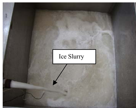
Fig.3.23 Photograph of Ice Slurry flowing in tank
