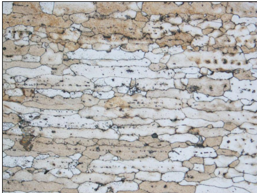
Fig 5.62: Microstructure of HAZ of welded AA7039 (100x)
