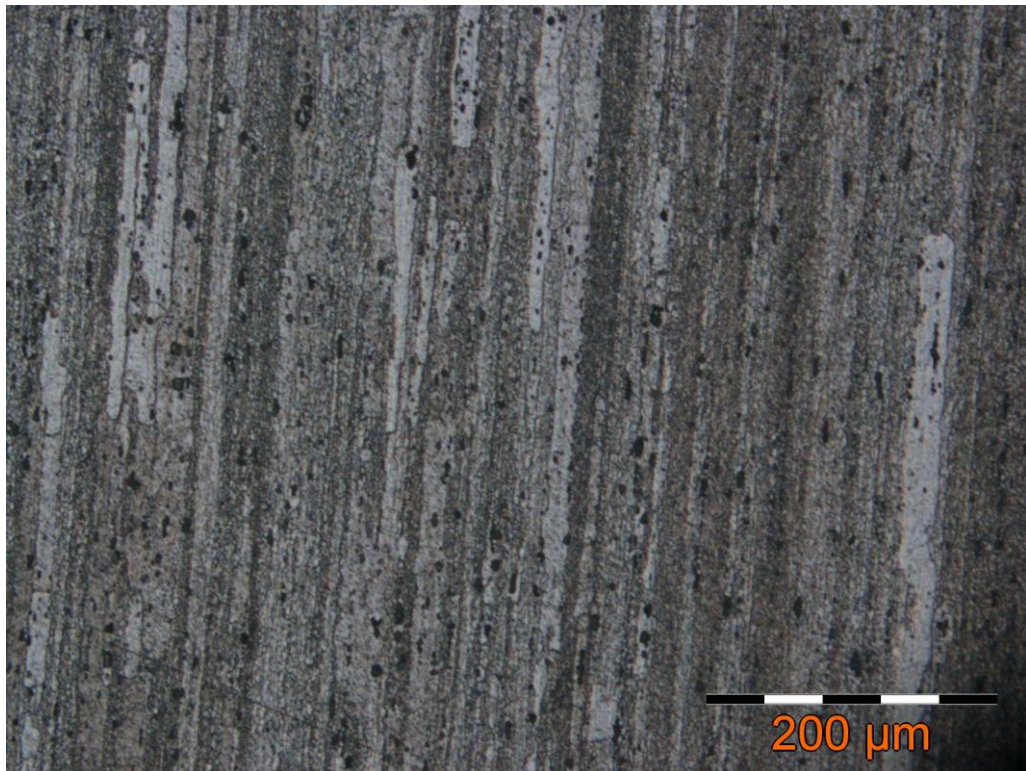
Fig 5.19: Microstructure of Base Metal of Al Alloy 7039
