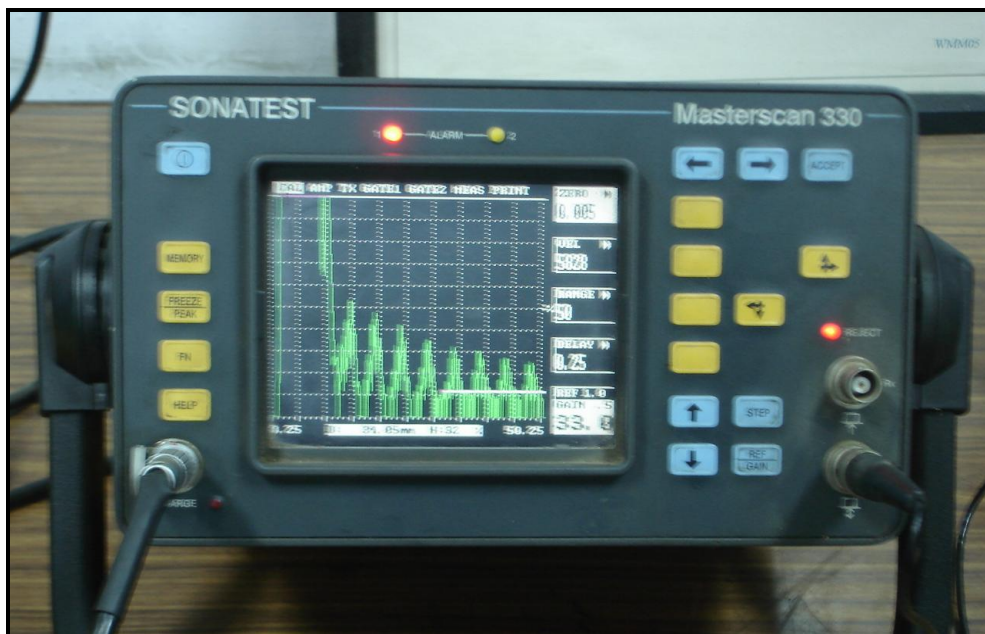
Fig 3.13: Digital Ultrasonic Flaw Detector (Test Range – Up to 10 m in steel, Test Mode – Pulse Echo, Frequency range – 1.5 to 10 MHz)
