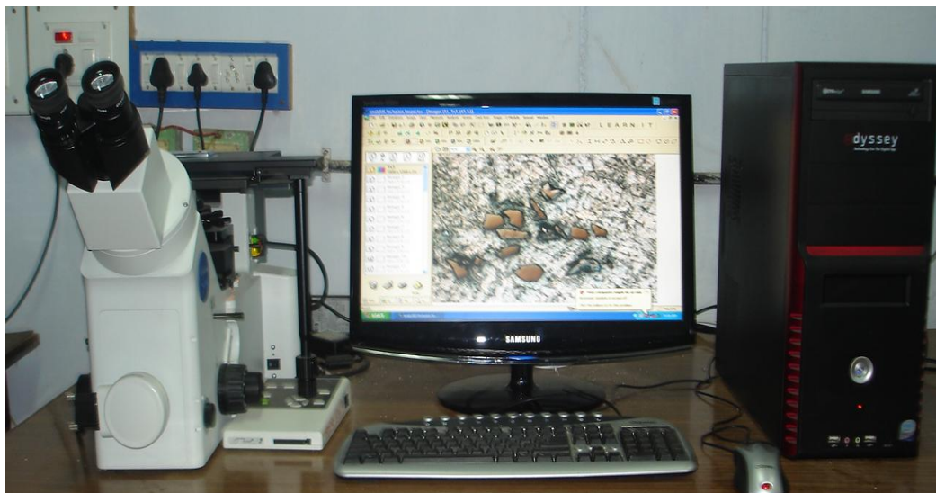
Fig 3.15: Metallurgical Microscope with Image Analyzer Software (Make – Olympus Corporation Japan, Magnification – 50X TO 1000X, Image Analyzer Software – Inclusion inspector)
