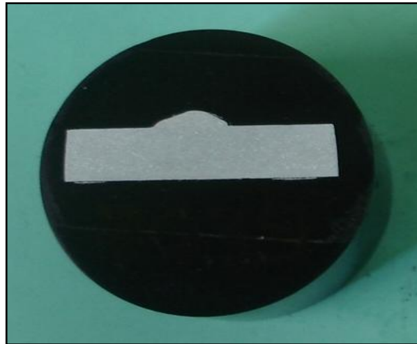
Fig 3.6: Mould Sample for Bead Geometry Measurement and Microstructural Analysis
