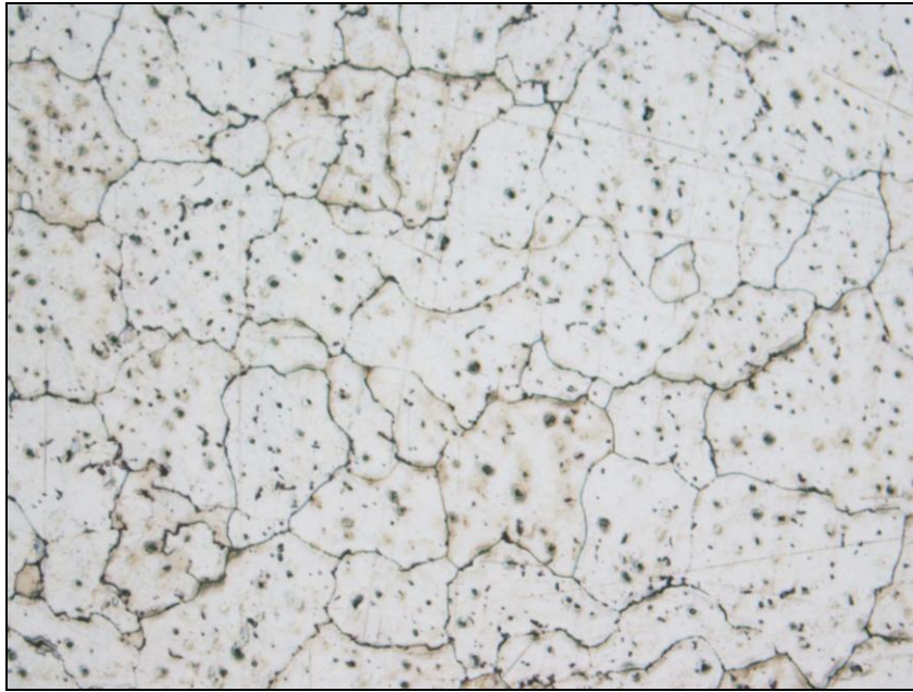
Fig 5.64: Microstructure of welded AA7039 at Weld Zone
