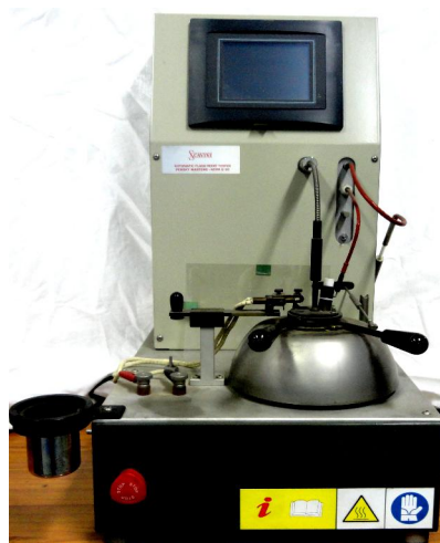
Fig. A3. A Pensky Martens apparatus used for determination of flash point Calorific Value
