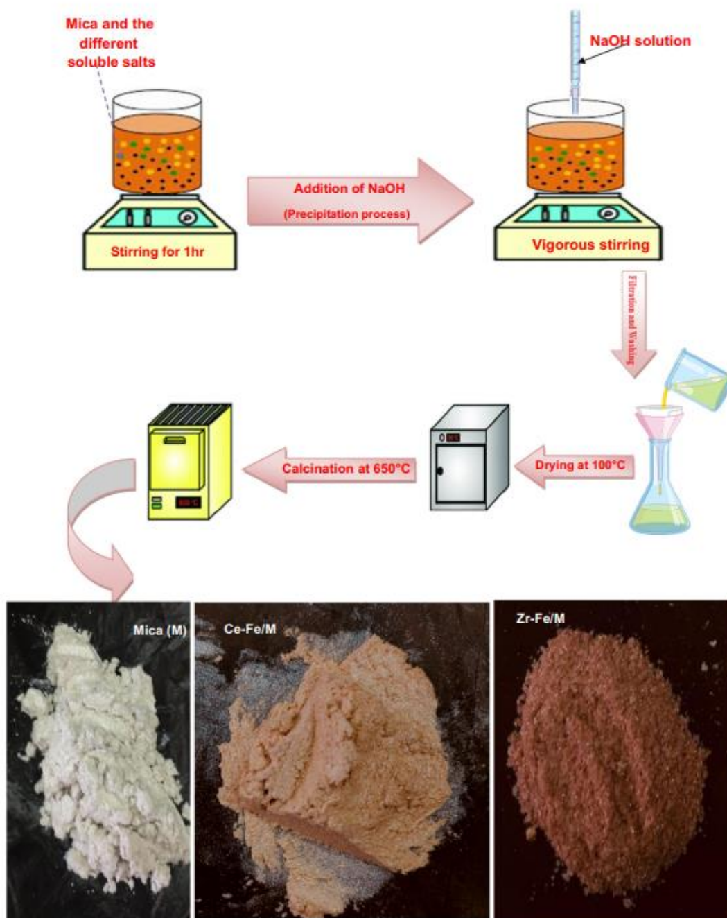
Figure 6: Preparation process of oxide coated mica pigments. [59]
