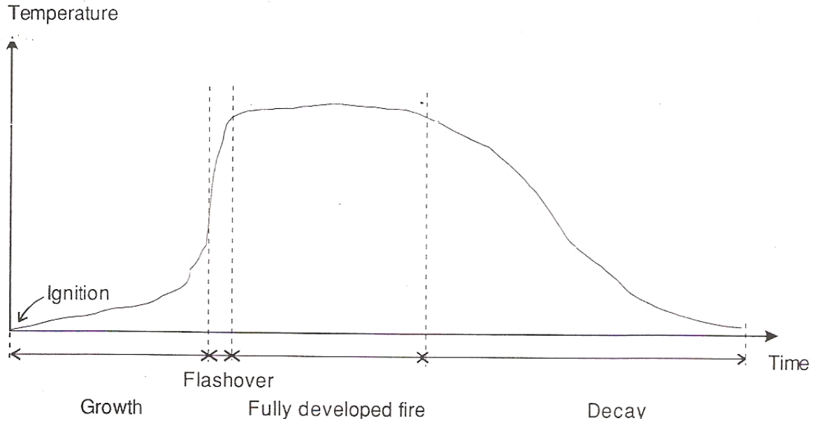
Fig. 1.12 Idealized description of the temperature variation with time in an enclosure fire.
