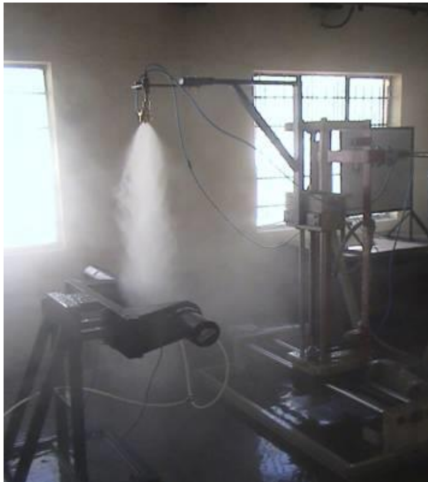
Fig. 4.6 Characterization of Atomizer for Droplet Size Measurement
